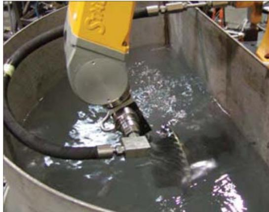
*Cavitation peening is used to generate compressive residual stresses in metals and ceramics*
