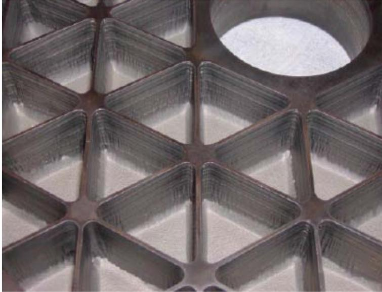
*Ormond milled 1-inch deep pockets in delicate CVD silicon carbide material for optical components for space applications*
