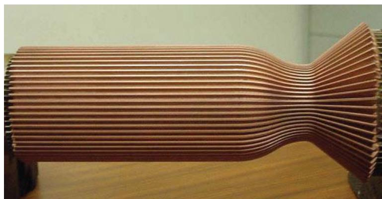
*Abrasivjet milling applications addressed by Ormond range from space optics to tiny heat exchangers and rocket combustors.*
