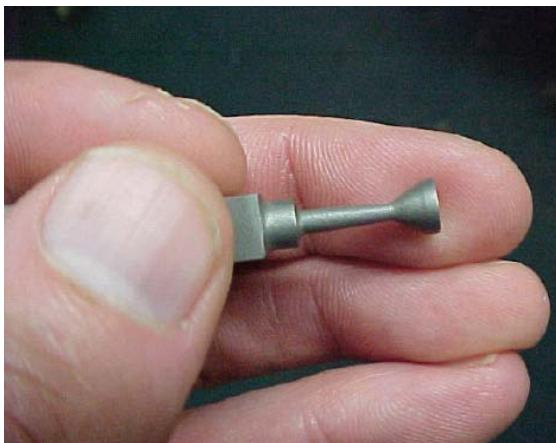
*Abrasive waterjet turned rhenium valve pintle machined to within 0.001 inch*
