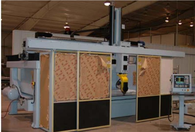
*High performance custom tooling is designed and built at Ormond to meet special requirements (6-axis machining center shown)*
